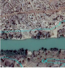
Figure 4. The Sirba flood line at Tallé according a 100 years (white) and a 20 years (light blue) return period.
